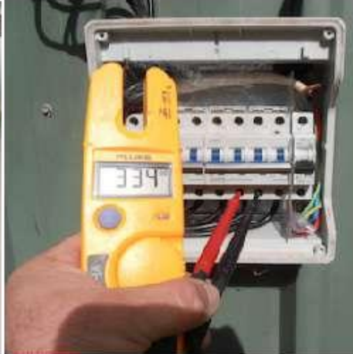
Fig. 9.3.5 Checking of reverse polarity using a clamp-on meter (Voltmeter)
