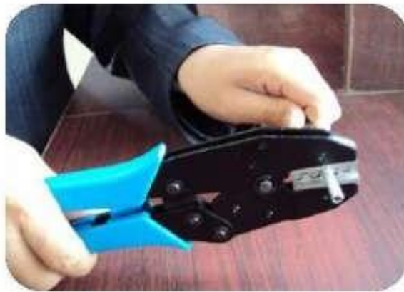
Fig. 8.3.5 Cable stripping by using crimping tool
