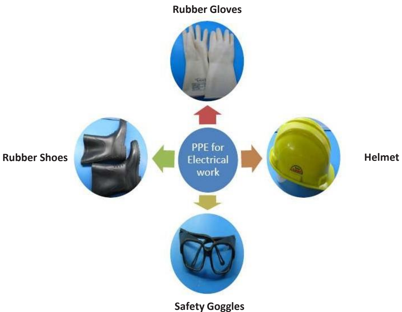
Fig. 8.1.2 Personal Protective Equipment (PPE) for Electrical Work
