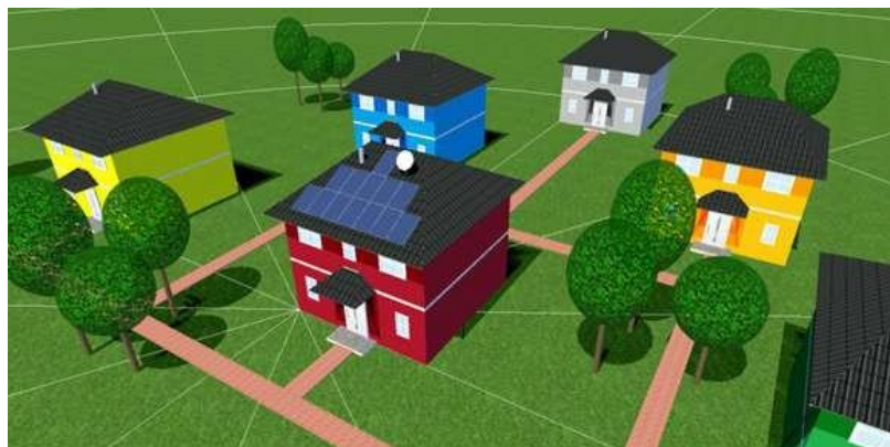
Fig. 5.1.5 PV array installations must be carried out after thorough consideration of possible shading objects surrounding the location
