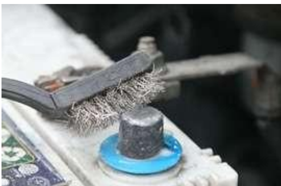
Fig. 10.2.11 Cleaning of batteries terminals to avoid corrosion and loose connections
