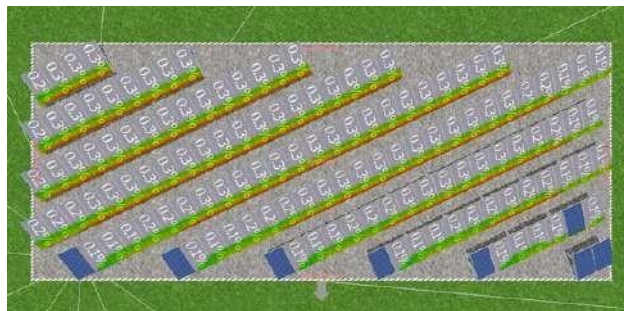
Fig. 5.3.13 Detailed shading analysis - Effect of shading on individual solar modules
