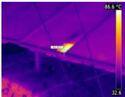
Fig. 9.3.1 Spot shading causes hot spot and may damage a module
