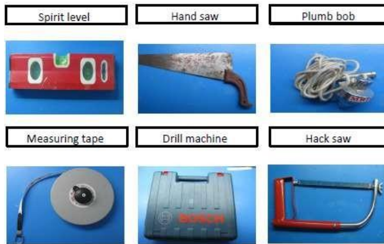
Fig. 7.1.3 Tools and Tackles for Civil/Mechanical work
