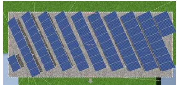
Fig. 5.3.12 3D modelling of rooftop solar PV system
